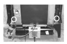
13) Connect long black & red wires to thermodisc and secure wires.
